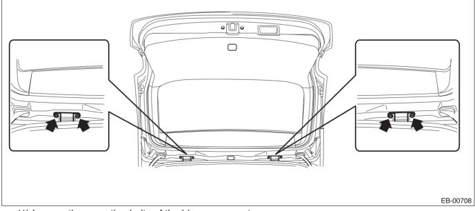
(1) Loosen the mounting bolts of the hinge - rear gate.
