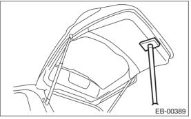
2) Remove the mounting bolts and remove the stay assembly - rear gate.
