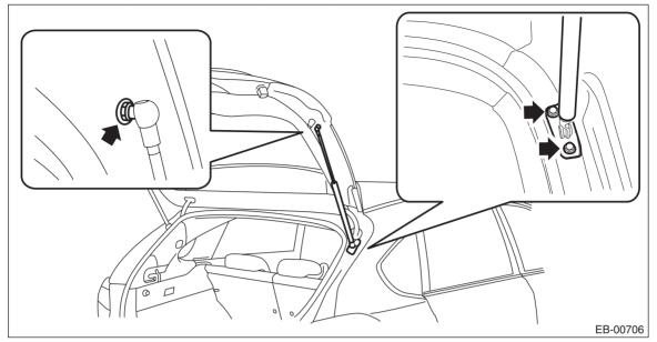
14) Remove the bolts of the hinge - rear gate, and remove the panel - rear gate.
