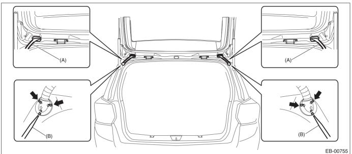
10) Pull out the harness and the hose assembly - rear washer from the panel - rear gate.
