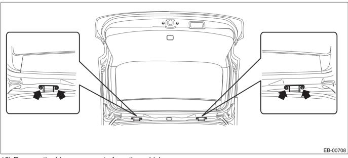
15) Remove the hinge - rear gate from the vehicle.
